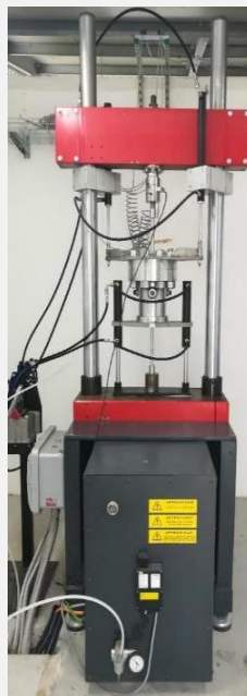
Vertical servo-mechanic Italsigma SSRT testing frame equipped with 1000 bar vessel for hydrogen application.
