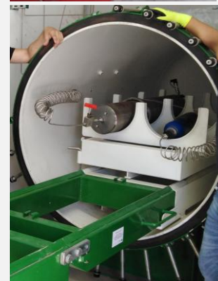
Vessels ready for test, placed into the safety chambers and loaded samples placed into the vessel
